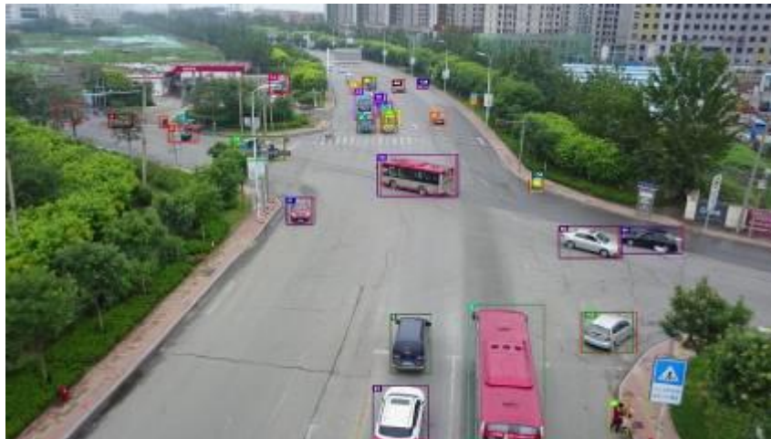
Figure 6. Sample frame with tracking results of one the sequences of the VisDrone 2018 dataset. Numbers stand for the identifiers of the tracked vehicles.
